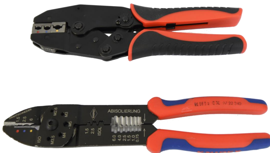
Proper tools for crimping.
