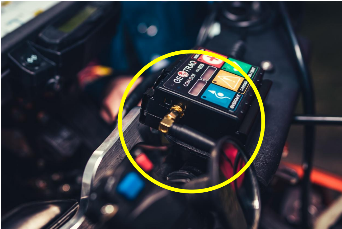
Installed antenna on the Com-Box unit.
